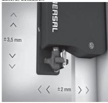
The axial misalignment (Y) is max.  $\pm$  3.5 mm. The height misalignment (X) is max.  $\pm$  2 mm.
