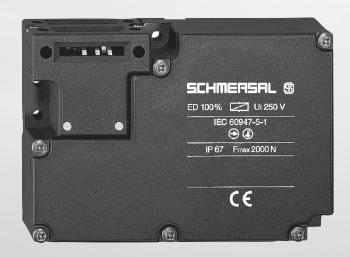
Solenoid locking switches are used on sliding, hinged and removable guard doors that must be closed and locked for operator safety. It is a two part system consisting of a switch body, mounted to the guard frame, and a separate actuator key, mounted to the door.
