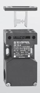
Keyed interlock switches are used on sliding, hinged and removable guard doors that must be closed for operator safety. It is a two part system consisting of a switch body, mounted to the guard frame, and a separate actuator key, mounted to the door.
