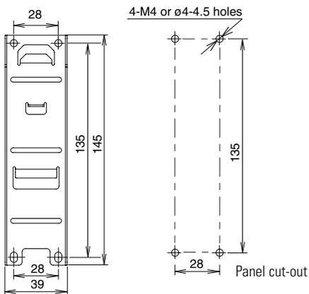
When a PS9Z-6R1F is installed on PS6R
