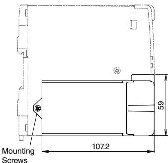
When using a PS9Z-6RS1 Branch Terminal Unit
