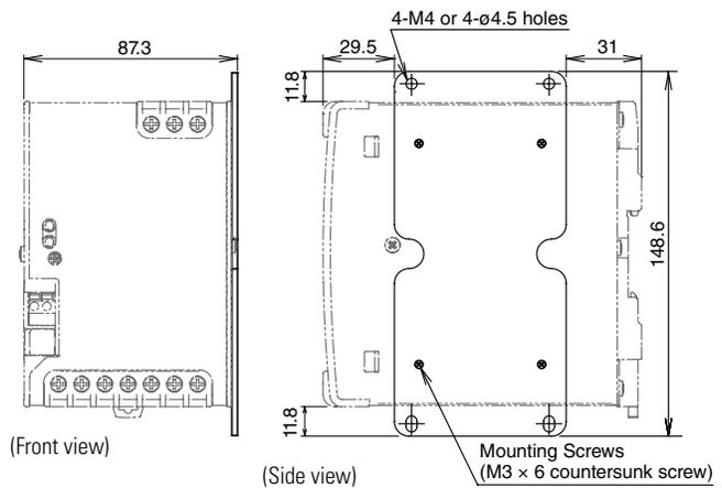
When using a PS9Z-6RM\* DC-DC Converter Unit
