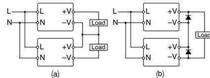
Select a Schottky diode in consideration of the rated current. The diode's reverse voltage must be higher than the PS6R's output voltage.
