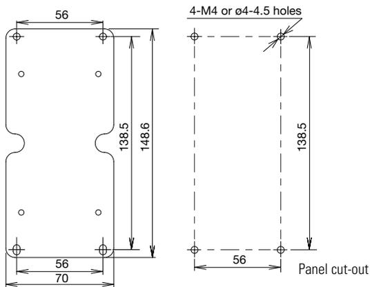
When a PS9Z-6R2F is installed on PS6R
