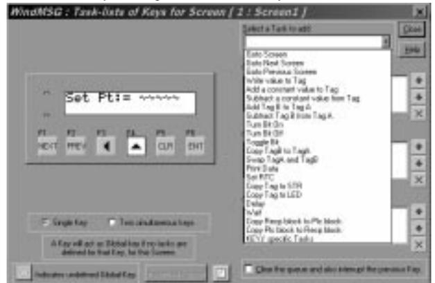
Select Turn bit on task as 'press task' for the key.
