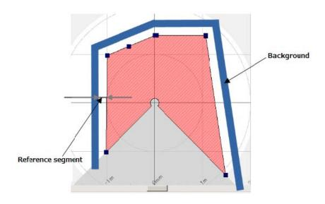
Figure 3-7 Protection zone configured using teaching mode
