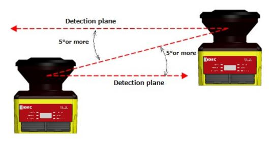
Figure 5-3 Parallel installation
