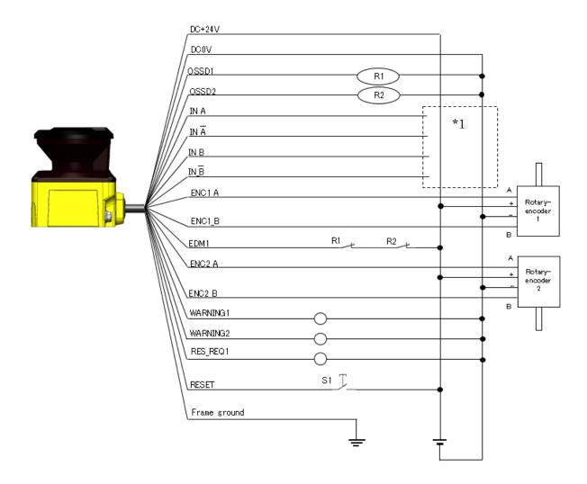
Figure 6-3 Wiring Example 3
