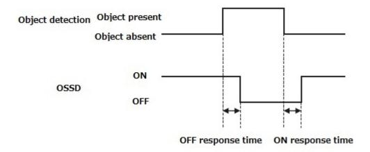
Figure 3-15 Timing chart of automatic restart
