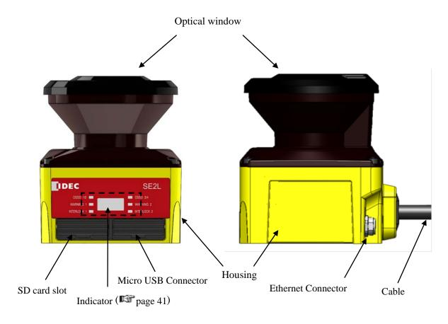
Figure 3-1 SE2L-H05LP / SE2L-H05LPC components
