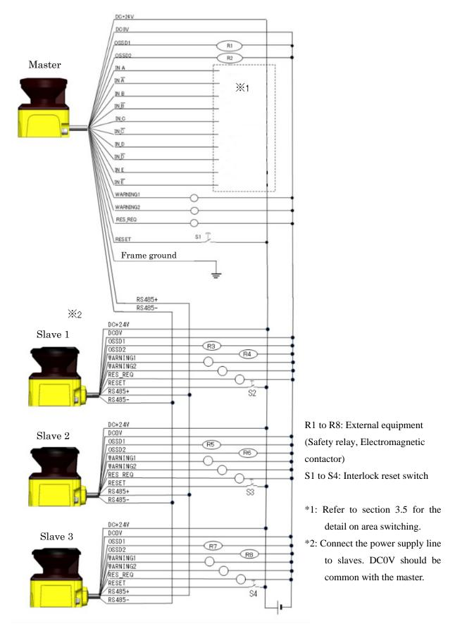
Figure 6-5 Wiring Example 5
