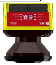
Figure 3-27 Example of upside-down configuration (The area number is 02.)
