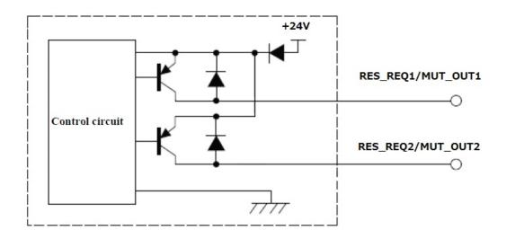
Figure 6-7 Output circuit
