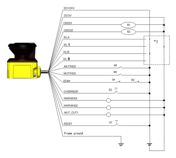
Figure 6-2 Wiring Example 2
