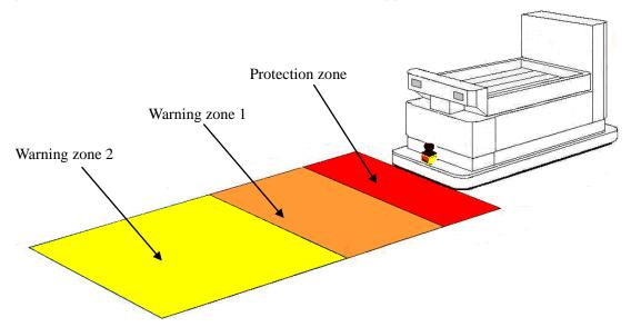
Figure 4-10 Example of area protection (Mobile)
