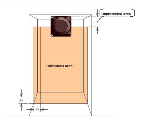
Figure 4-6 Top view of access protection (Whole body detection)
