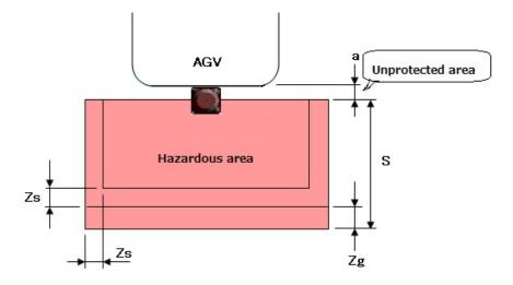
Figure 4-11 Top view of area protection (Mobile)
