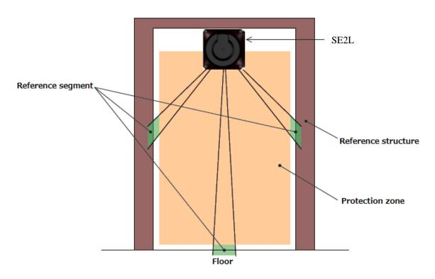
Figure 3-23 (c) Incorrect configuration of reference segment
