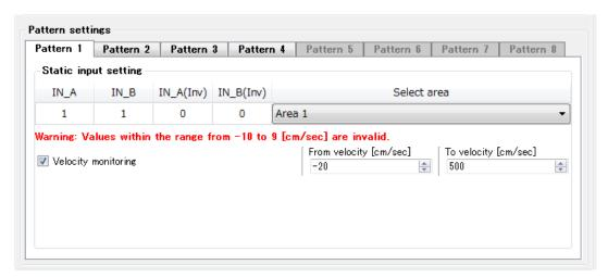
Figure 3-13 (b) Example of static input setting
