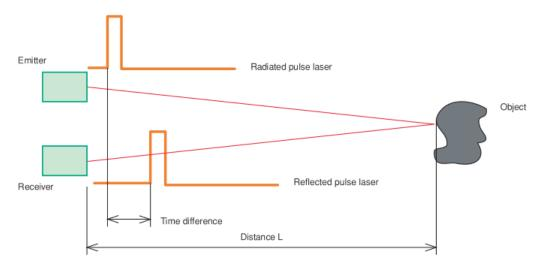
Figure 3-5 TOF operation principle
