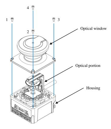
Figure 8-1 Remove the optical window
