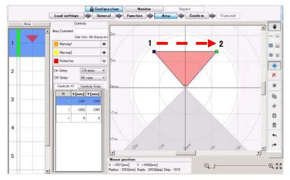
When a straight line is drawn from point  $1 \rightarrow$  point 2, a triangular shape is formed by connecting these two lines with origin. Coordinates of point 1
