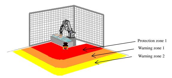
Figure 4-1 Example of access protection
