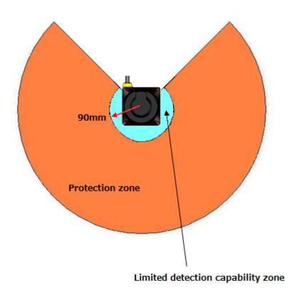
Figure 5-9 Limited detection capability zone
