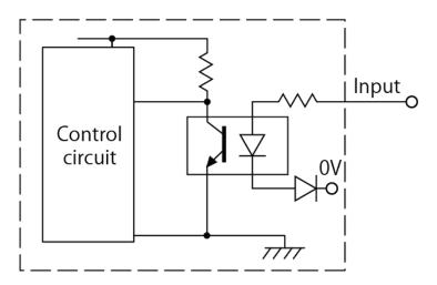
Figure 6-8 Input circuit
