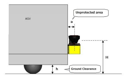
Figure 4-12 Side view of area protection (Mobile)
