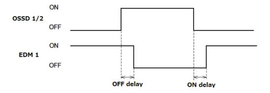
Figure 3-19 EDM timing chart
