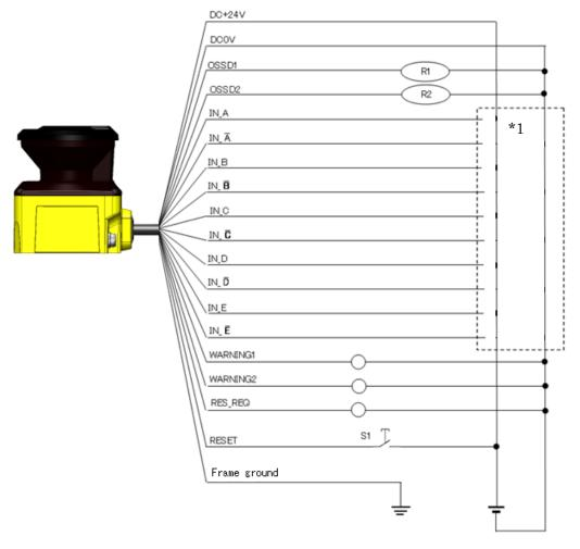
Figure 6-1 Wiring Example 1
