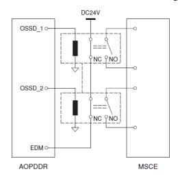
Figure 3-18 EDM circuit
