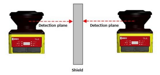
Figure 5-7 Parallel installation
