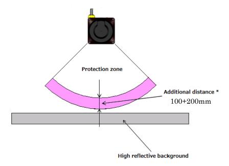
\* Additional distance : Required additional distance when operating SE2L under high reflective background Specification of Distance tolerance is "+100mm".
