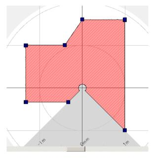
Figure 3-6 Protection zone configured using manual mode
