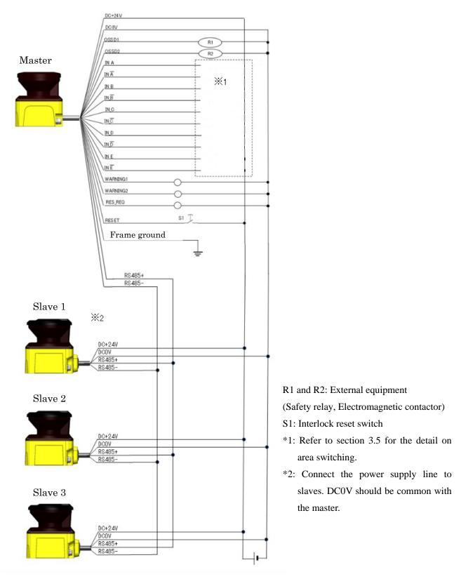
Figure 6-4 Wiring Example 4
