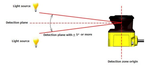
Figure 5-1 Installation to avoid light interference
