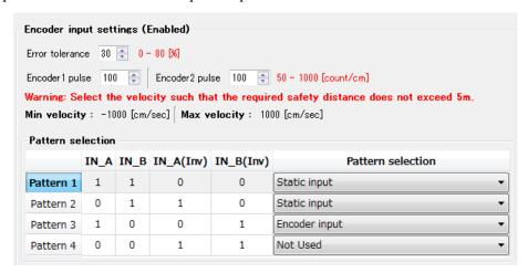
Figure 3-12 Example of pattern switching through encoder input
