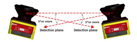
Figure 5-5 Parallel installation
