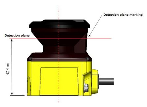
Figure 3-3 Detection plane of SE2L-H05LP / SE2L-H05LPC (Side view)
