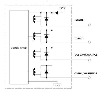
Figure 6-6 OSSD/WARNING Output circuit
