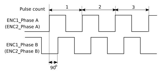
Figure 3-10 Input signal through Incremental encoder
