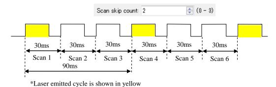
Figure 3-31 Operation of SE2L when scan skip count is 2
