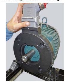
6.0 Position the wheel such that its front surface is flush with housing groove surface.
