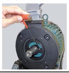
10.0 Pull the mating connector out and complete wiring per electrical connections table
