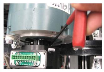
Tighten the collar clamp to stated torque provided on the encoder datasheet (50-55 in-lbs).
