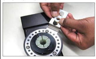
Slide the flat nylon washer one the side away from the bend and the flanged nylon washer on the side of the bend and press them together until they are fully seated in the tether slot or hole. One steel washer is to be used on each side of the nylon washer (step 6).
