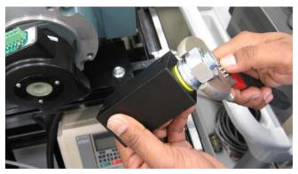
Loosen the conduit fitting nut to guide the cable through it and then fully tighten the nut.
