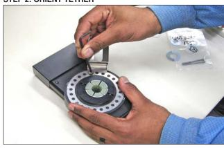
Rotate the tether to the required orientation and tighten the tether to the encoder body using three #10-32 screws provided. The hollow-shaft series encoder tether can be rotated in 15 degree increments so that connector or cable exit can be conveniently located.
