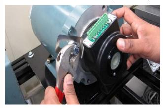
Rotate the tether arm until it is at the correct orientation and is aligned with the mounting holes on the motor or equipment. Install one steel washer on both sides of the nylon washer. Fasten the tether arm to the motor housing using the supplied bolt. Ensure that there is no stress or flexing of the tether arm when secured.
