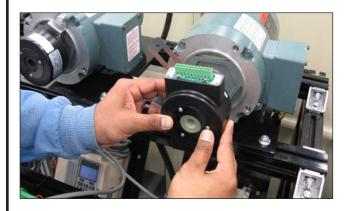
Carefully slide the encoder all the way down until the tether rests on the motor face without any stress on the tether. Do not tighten the shaft clamp on the encoder yet.
