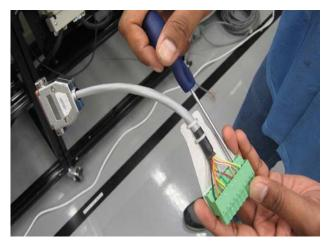
Prepare the cable by connecting it to the plug connector component per the electrical connection table provided on the encoder datasheet.
