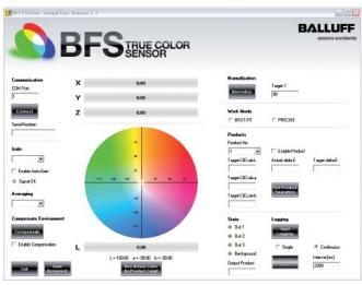
Configuration is easy and intuitive with software. The Lab color values are transmitted via this interface to set the tolerances of the outputs.
