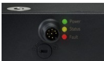
3 color LEDs for signaling: Green = Power; Yellow = Status Red = (Flashing) Diagnostic error
