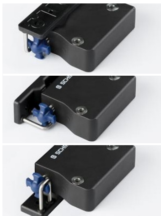
External cam allows actuator to approach from three directions for mounting options. Same unit can be mounted for left or right hinged doors.
