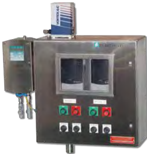
Install AC drives in the hazardous area with Bebco EPS 6000 purge and pressurization enclosure. High ambient temperature can use a vortex cooling system for temperature control.
