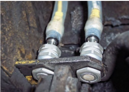
PTFE coated Prox-Mounts and Weld Repel® tubing over sacrificial cables improve sensor life and productivity.
