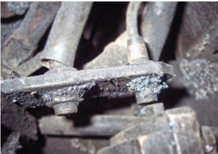
Slag accumulation and unprotected pigtail sensors cause large amounts of downtime.
