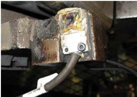
Standard sensors can accumulate slag, damage the sensing face and cause false tripping of the sensor.
