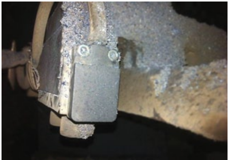
Steelface® sensors with W51 ceramic coating resist the slag and the sensor can be brushed clean with no damage or issues.
